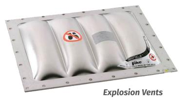
Venting is the most commonly used method to protect dust collectors against destruction or deformation as a result of the excessive forces exerted by explosion pressure. Explosion vents are designed to protect the dust collector from overpressure of deflagration. Vent opens at a constant pressure to prevent the pressure increase inside the dust collectors. Dust collector and venting area has to be at a safe area.
